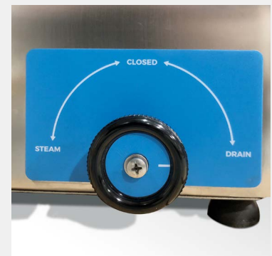
Detail of the 3 position manual valve installed in both AES-8 and AES-12.
