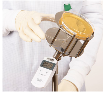
2. POSITIONING OF THE OPEN CULTURE PLATE ON TOP AND THE LID ON BOTTOM OF TRIO.SETTLE
