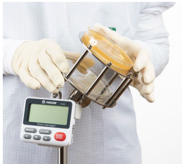
Articulate table and floor stainless steel support for Passive Air Sampling
